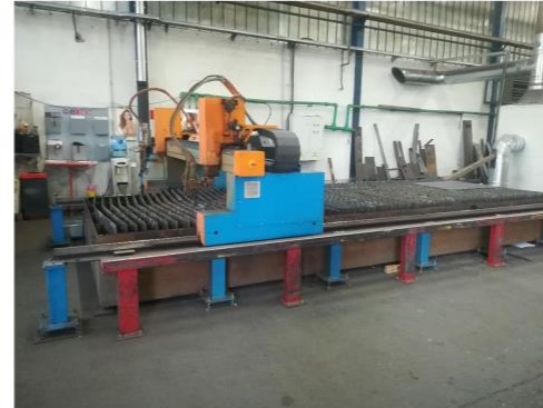
Hypertherm MAX PRO 200- CNC plasma cutting system
