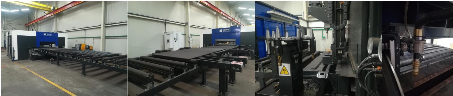
Vernet Behringer: MAG evo 620- CNC Plasma cutting, drilling, punching...
