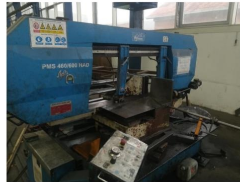
Pilana pms 460-600 had- Band Saw- for pipes-carbide blade
