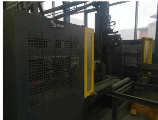
Ficep 901 db: Automatic CNC drilling and sawing line
