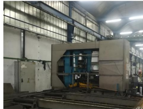
Vernet Behringer: FP600,HBP360- CNC Beam saw drill
