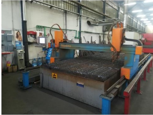
Hypertherm MAX PRO 200- CNC plasma cutting system
