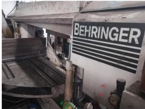
Vernet Behringer: FP600,HBP360- CNC Beam saw drill
