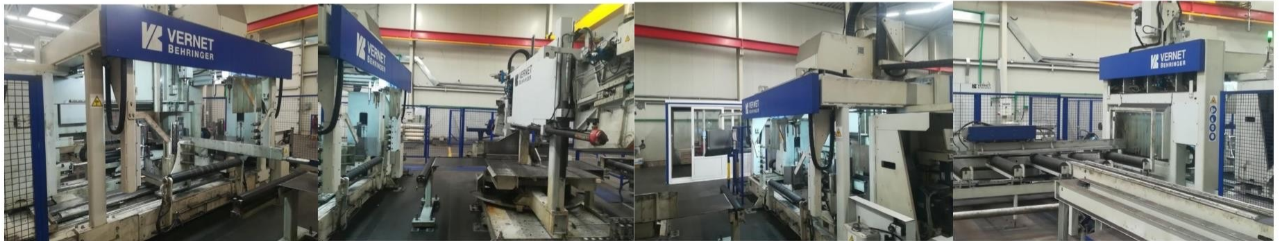
Vernet Behringer: HD-X evo 1218- CNC Beam line machine
